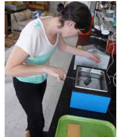
Hot water seed treatment with a precision hot water bath. Photo: UMass Extension
